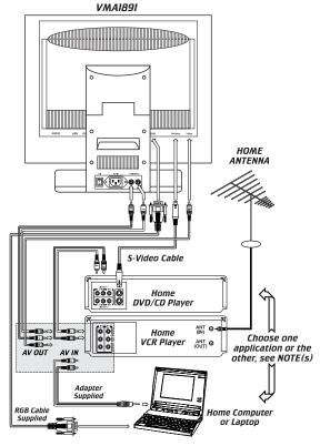
NOTE: Since there is only one set of L/R audio inputs on the VMA1891, additional components must route their audio signals through the VCR A/V inputs. This may limit the components attached to the VMA1891.
